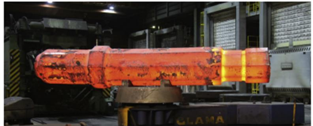
HP rotor at final forging, COST steel E.
