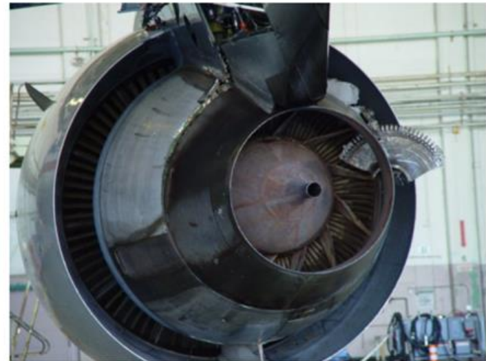
Figure 3. View of the exhaust of No. 2 engine showing piece of HPT stage 1 disk protruding from the right side of the engine exhaust duct.
